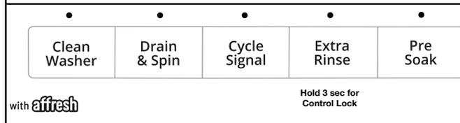
To add an option to the cycle, touch its name – Extra Rinse. To remove an option from the selected cycle, touch that button again.
