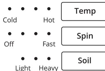
The led indicator lights will show the default settings for the selected cycle. To adjust a setting, touch its name – Temp, Spin, or Soil. Adjusting settings may change the Estimated Time Remaining. Tightly packing the load, unbalanced loads, or excessive suds may also cause the washer to increase the cycle time.
