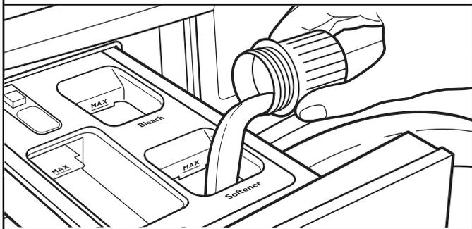
Pour a measured amount of liquid fabric softener into liquid fabric softener compartment. Always follow manufacturer's directions for correct amount of fabric softener, based on your load size.
