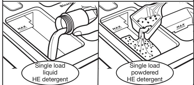
Adjust the selector, based on type of HE detergent used (either liquid or powdered). Add a measured amount of detergent directly into the detergent compartment. See the "Using the Dispensers" section.
