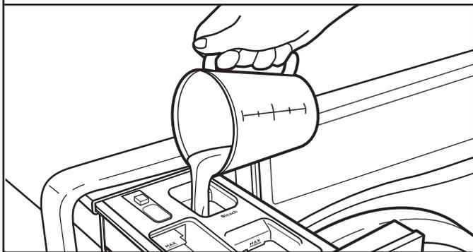
Add liquid chlorine bleach to the bleach compartment. Do not overfill, dilute, or use more than 2/3 cup (165 mL). Do not use color-safe bleach or Oxi in the same cycle with liquid chlorine bleach.
