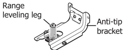
To check if the anti-tip bracket is installed properly, use both arms to grasp the rear edge of the range back. Carefully attempt to tilt range forward. When properly installed, the range should not tilt forward.
