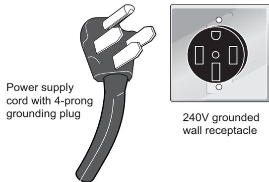
It is the personal responsibility of the consumer to have the appropriate outlet with the correct, properly grounded wall receptacle installed by a qualified electrician.
