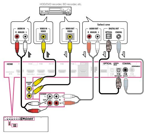
In order to record, you must connect the analog audio cables (the digital connection is for playback only) (page 64).
