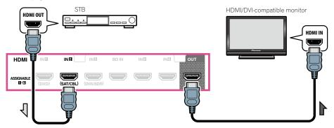
• Even if your set-top box is equipped with an HDMI output terminal, in some cases the sound is output from the digital audio output (optical or coaxial) and only the video is output from the HDMI output terminal. In this case, make the HDMI and digital audio connections as shown below.
