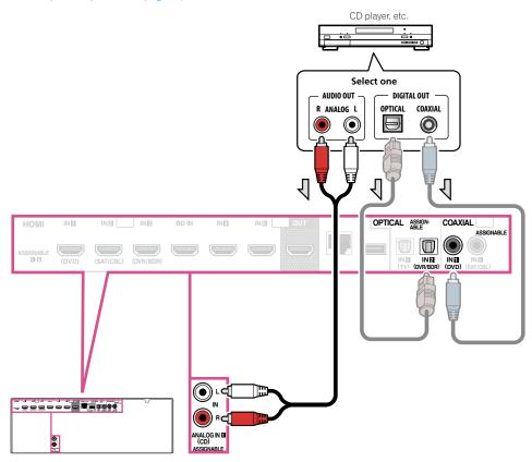
If your turntable has line-level outputs (i.e., it has a built-in phono pre-amp), connect it to the ANALOG IN 1
