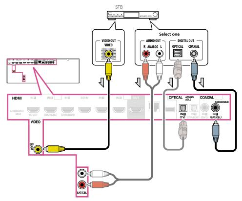
If your set-top box is equipped with an HDMI output terminal, we recommend connecting it to the receiver's
