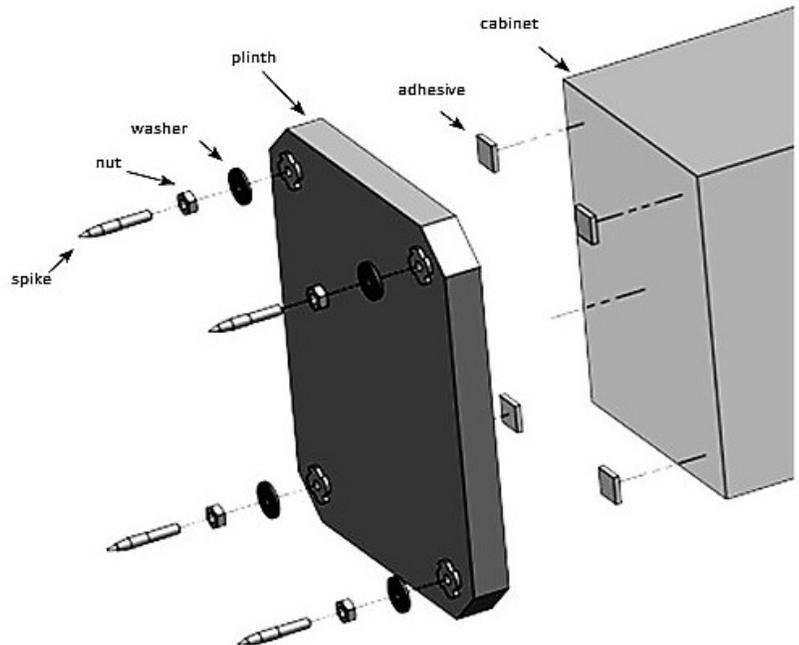
Thread a nut onto the spike. Next, slide a silicone washer into the spike assembly. Insert the assembly into the plinths. Repeat this procedure until all 8 spikes are fastened into the plinths. Once all the spikes and washers are installed level the plinth to the floor.
