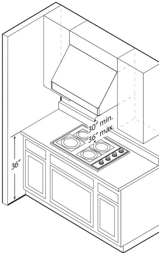
Minimum mount height between range top to hood bottom should be no less than 30".
