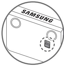
You can turn the sound sensor on or off by using its button at the bottom of the TV.
