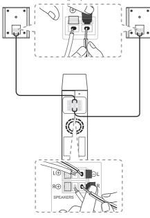
2. Connect the wireless receiver and the rear speakers (right, left) with the speaker cables.
