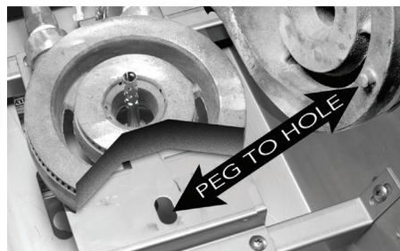
3. Ensure that the burner is seated correctly on the frame, with the brass peg seated inside the positioning hole.
