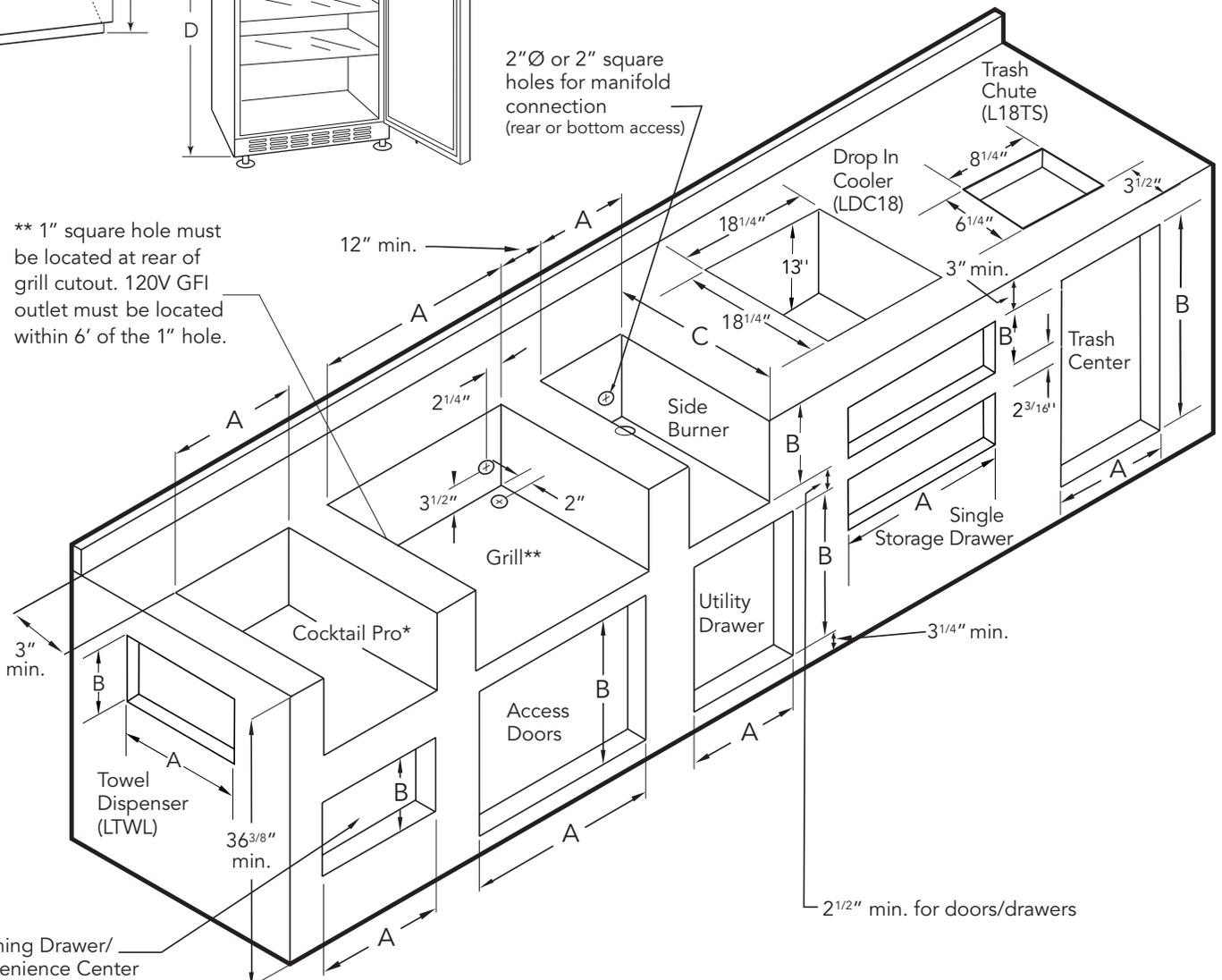
\* Cocktail Pro should have an open bottom for plumbing and drain access.
