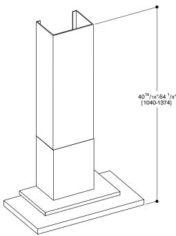
Suitable for ceiling heights of 8.7 ft. (2.64 m) to 9.7 ft. (2.97 m); Specifications refer to a distance from floor to lower duct cover edge of 5.2 ft. (1.60 m).
