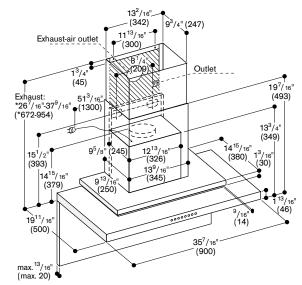
Suitable for ceiling heights of 7.4 ft. (2.27 m) to 8.4 ft. (2.55 m); Specifications refer to a distance from floor to lower duct cover edge of 5.2 ft. (1.60 m).
