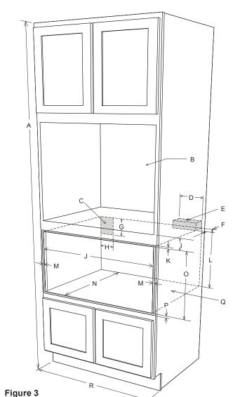
Figures 1, 2 and 3 contain the appliance and cutout measurements for reference when planning the drawer's
