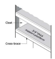
Mounting platform must be <sup>3</sup>/4" (1.9 cm) thick and able to support 100 lbs. (45.4 kilos)
