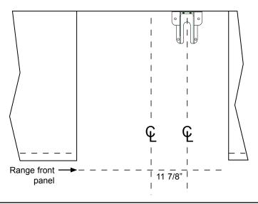
5. Place the bracket against the wall in the mounting location. Using a 1/8" bit, drill four 1-5/8" deep pilot holes perpendicular to the screw-seating surfaces shown below. Attach the bracket to the wall as shown with the included #12 x 1-3/4 screws.
