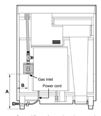
Gas and Power Access (panels removed to show gas connections)
