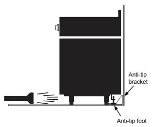
5. Use a level to confirm that the range is parallel to the ground and stable. Re-adjust the legs and change the height if necessary. Make sure the range does not tip or lean.
