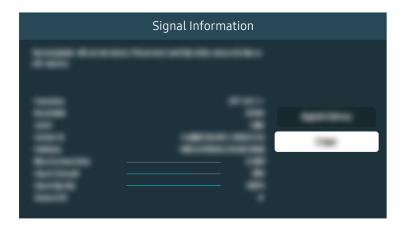
Signal strength must be more than 20 dB (more than four bars on the icon) for stable signal reception.
