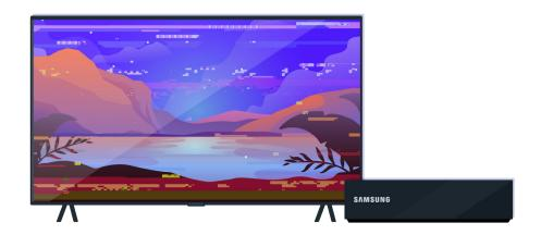
Check the antenna and input cable connections.
