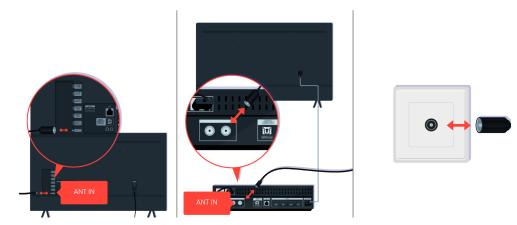
Check the antenna and input cable connections.
