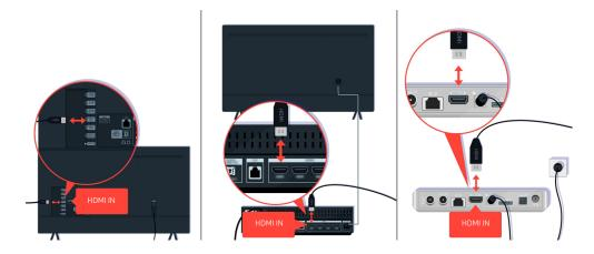
Check the antenna and HDMI cable connections.
