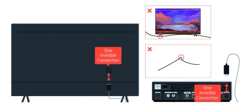
If the problem persists, and if your TV uses the One Invisible Connection, disconnect and reconnect the One Invisible Connection to the TV and the One Connect (OC) Box. Ensure that the One Invisible Connection is not pinched or bent sharply.
