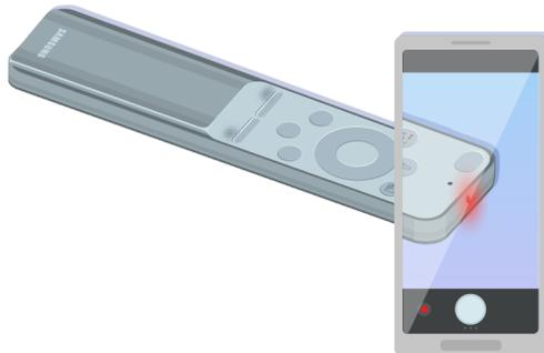
You can check whether the signal is being transmitted by pressing the power button and observing the front tip of the remote control through the camera on your smartphone.
