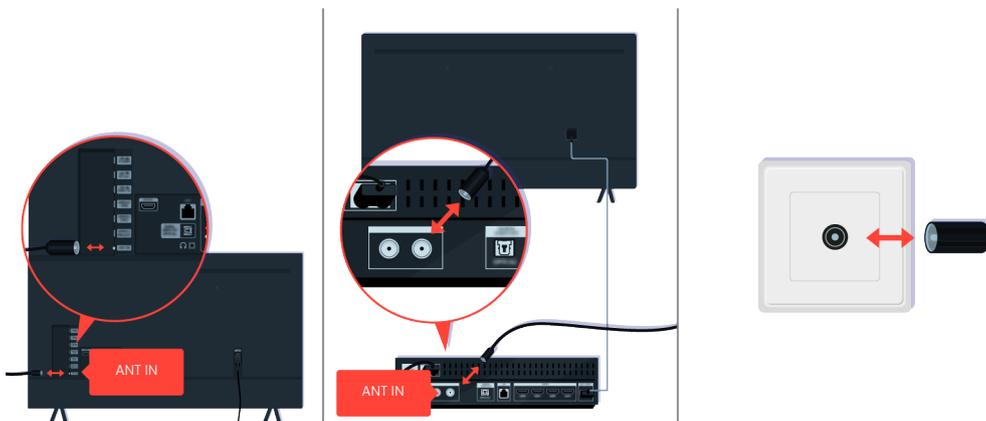
Check the antenna and input cable connections.
