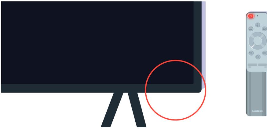
If the remote control sensor turns off when you press the power button, your TV is correctly connected to the power supply.
