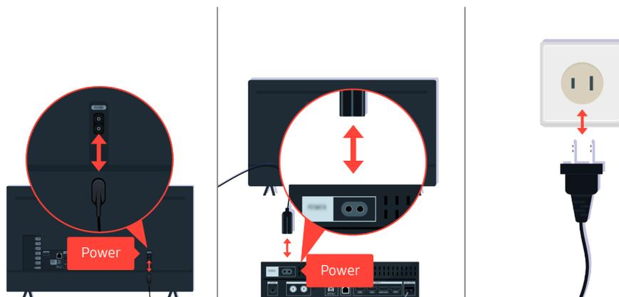
First disconnect and reconnect the power cables and HDMI cables on the back of your TV or the One Connect (OC) Box, then unplug the power cord and plug it back into the wall outlet.
