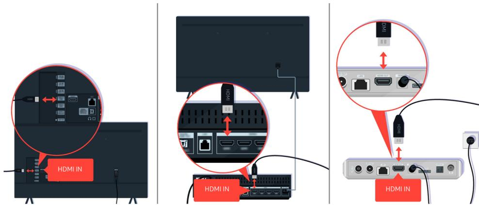
Check the antenna and HDMI cable connections.
