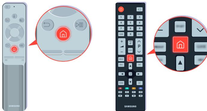
If the problem disappears during the test, check your TV signal. On the remote control, press the
