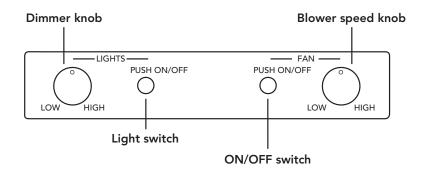
**ON/OFF switch**—Starts and stops the blower. When turned on the blower will operate at the previous setting of the speed control.
