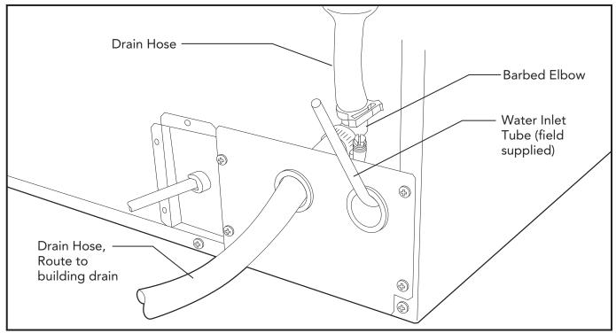
Back View, Gravity Drain Model
