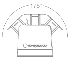
Bracket allows for 175° rotation on horizontal axis
