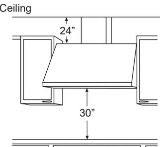
**9 ft Ceiling:** Install the hood 24" min. and up to a maximum of 30" above the cooking surface. The duct cover will expand to reach ceiling height.
