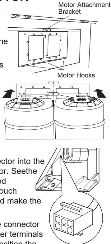
**IMPORTANT:** Hold the connector so the two square corner terminals are at the top as you position the connector to plug it in.
