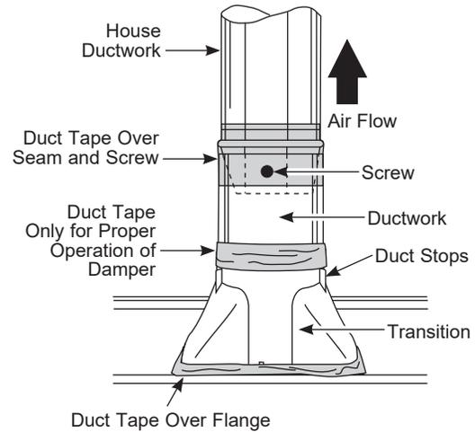
**CAUTION** Do not use sheet metal screws at the transition to ductwork connection. Doing so will prevent proper damper operations. Seal connection with tape only.
