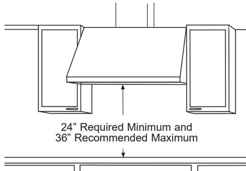
For this installation, a decorative duct cover is available to conceal the ductwork running from the top of the hood. Use of the duct cover requires special consideration to the installation height above the countertop. See page 12 for details.
