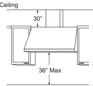
**10 ft. Ceiling:** Install the hood 32" min to 36" max. above the cooking surface. The duct cover will expand to a maximum of 34" above the top of the hood to meet the ceiling.
