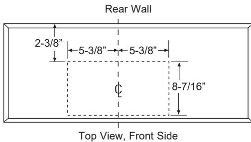
Cut a 10-3/4" x 8-7/16" hole through bottom of soffit or cabinet for duct transition as shown.
