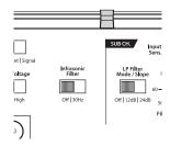
With ported enclosures and infinite baffle subwoofer systems, the use of the "Infrasonic Filter" is highly recommended to protect the speaker(s) from excessive excursion at inaudibly low frequencies.
