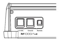
The M1000/lv2's "+12 VDC" and "Ground" connections are designed to accept 4 AWG power wire. 4 AWG is the required wire size for this amplifier.
