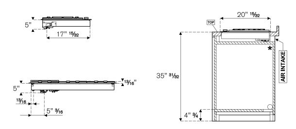
Bertazzoni recommends to operate the appliance after it has been installed in a cabinet. The kitchen cabinets shall be made of materials capable of withstanding temperatures at least 117°F (65°C) above room temperature in order to avoid possible damage to the cabinets during appliance usage. For further installation instructions refer to the installation manual.
