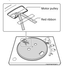
**3** Peel off the adhesive tape, pull and hold the red ribbon, and then hook the drive belt around the motor pulley.
