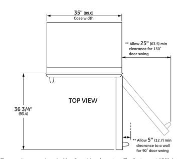
\*\*These units are equipped with a 2-position door stop. The factory set 130° door swing can be adjusted to 90° if clearance to adjacent cabinets or walls is restricted. Allow 15" minimum clearance to wall for pan removal. If the 90° door stop position is used, pan access is maintained but pan removal is restricted.
