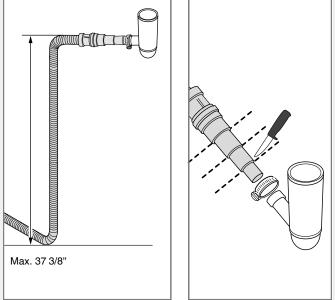
The drain hose can also be connected to a connection nipple on the sink unit's water trap. The connection nipple must have an internal diameter of at least 1/2".
