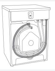
The machine is supplied with the outlet hose already attached. The hose should be extended over a suitable sink edge or drain pipe at a height of 24" to 36" (610 mm to 914 mm) above the bottom of the unit. (The lower height is preferable.) Make sure the hose is not kinked.
