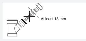
$\dot{\gamma}$  If the hose is extended, the internal diameter of the coupling must not be less than  $\frac{1}{2}$ .
