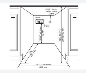
If the drain outlet is higher than 24"(610 mm), the connections will need to be recessed.
