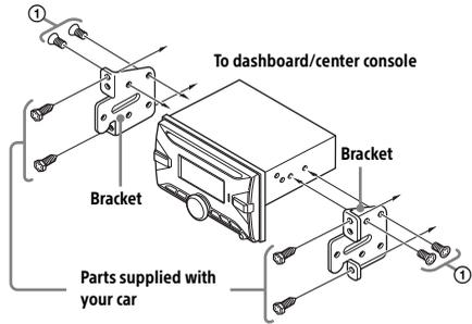
When mounting this unit to the preinstalled brackets of your car, use the supplied screws ① in the appropriate screw holes based on your car: T for TOYOTA and N for NISSAN.
