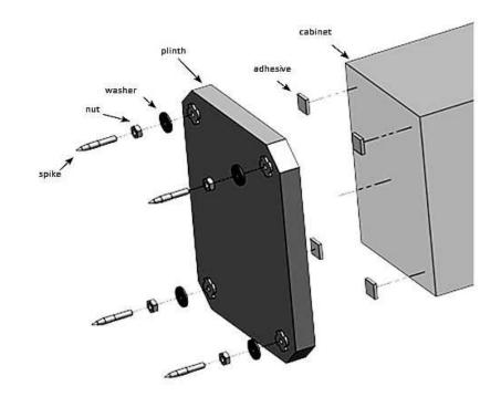
Thread a nut onto the spike. Next, slide a
