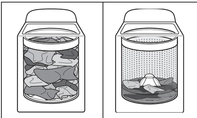
As the washer dampens and moves the load, the level of the items will settle in the basket. This is normal, and does not indicate that more items should be added.
