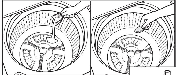
Add a measured amount of HE detergent or single-dose laundry packet into the basket. If using Oxi-type boosters, color-safe bleach, or fabric softener crystals, add to the bottom of the washer basket before adding clothes.
