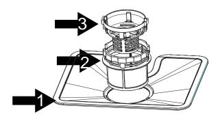
The filter system consists of a coarse filter, a flat (Main filter) and a micro filter (fine filter).
