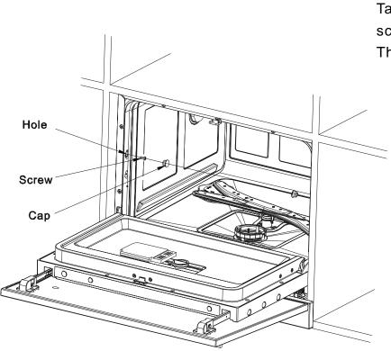
Step 6: Take out cap, a hole revealing, using screwdriver install screw, bothsides. Then recover the cap in hole.
