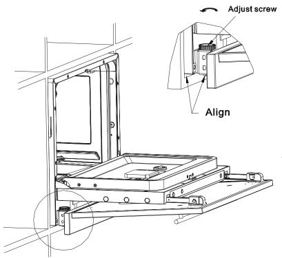
Step 5: Install the dishwasher in aperture, but not full, as figure, adjust screw, let its bottom align aperture's base, then push dishwasher full.
