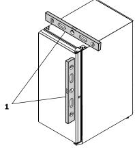
If the unit is not level, adjust the legs on the corners of the unit as necessary.
