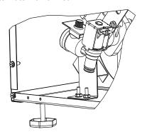
4. Break away filler feature in bushing with flat screwdriver.
