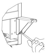
Remove corresponding screws on opposite side of cabinet.On some models there may be a nut behind one or both screws on either side.
