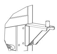
Remove corresponding screws on opposite side of cabinet. On some models there may be a nut behind one or both screws on either side.
