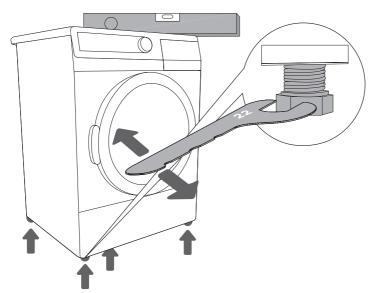
Level the dryer in longitudinal and traverse direction by rotating the adjustable feet which allow levelling by +/- 1 cm. Use key nr. 22 and spirit level.
