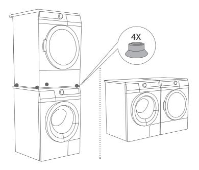
Positioning the appliance on top of the washing machine by using the vacuum feets or side by side.
