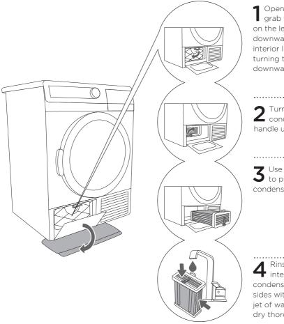
Open exterior lid, grab the handle on the left and pull downwards. Remove interior lid by turning the handle downwards.
