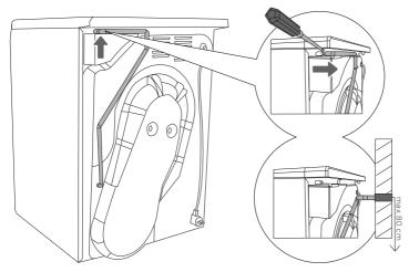
Pull the tube to remove it with flat screw-driver, from the holder on the appliance back wall.(on the left hand side under the cover).
