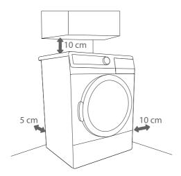
Ventilation slots and the opening on the front and rear side should always be kept free.
