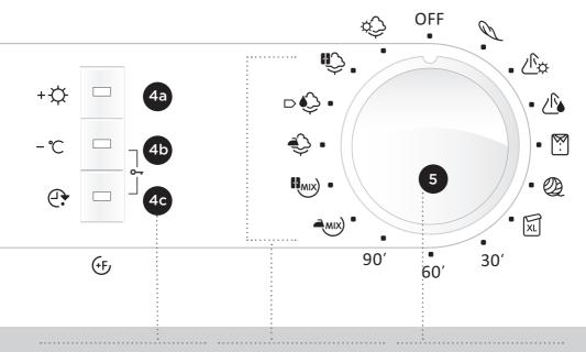
a, b, c: ADDITIONAL FUNCTION keys, to extend or adjust the basic programs.
