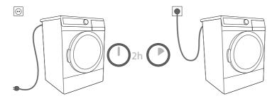
The dryer should be left to stand still for at least two hours before it is connected to the power mains to allow the system to stabilize.
