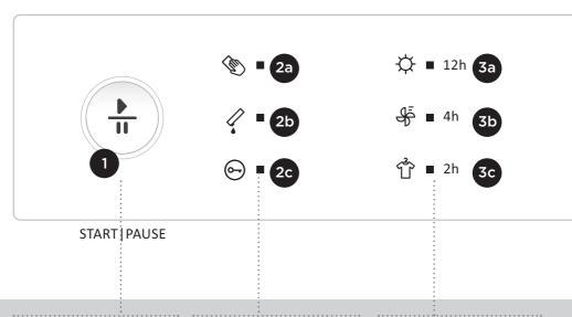
**1** START/ PAUSE key, use this key to start or stop the program. When selected, the signal light on the key will flash. When the program has started it will be lit continuously.
