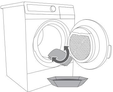
Clean the dryer drum before using the dryer for the first time. Use a damp cloth and a mild cleaning agent.
