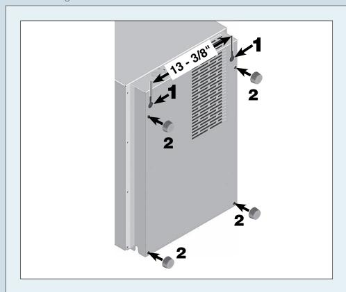
The appliance can be wall-mounted. There are two mounting holes **1** at the back of the appliance.
