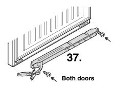
**37.** Turn soft stop mechanism through 180° and re-fit on the opposite side.
