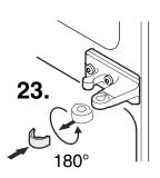
23. Remove hinge bushing, turn through 180° and re-fit.
