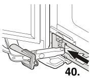
**40.** Slide door cover over soft stop mechanism hinge.
