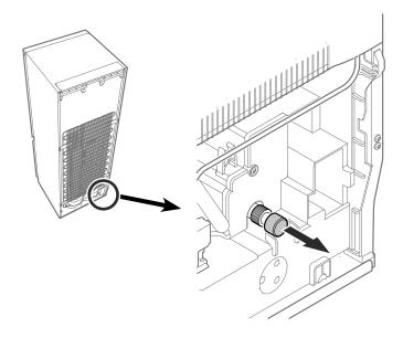
5. Screw the adapter onto the solenoid valve.
