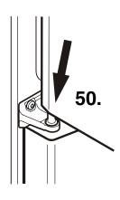
50. Suspend top door on hinge pin. For this, the door must be open at least 90°.
