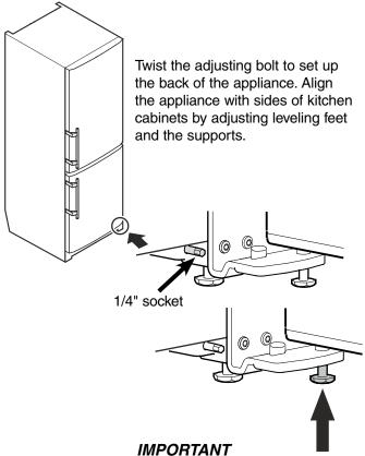
After final installation, this screw must be turned down until it has proper floor contact to support the hinge bracket.
