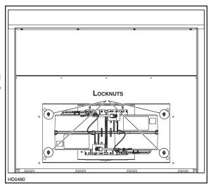
Refer to the instructions included with the selected blower/rough-in kit (sold separately) for details on installing the rough-in plate. Install the rough-in plate so that the wiring box is located on the right side as you are facing the hood.
