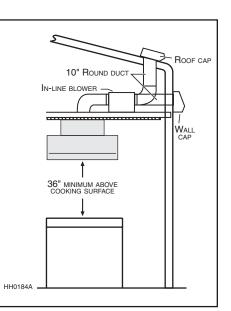
MODEL ILB11 IN-LINE BLOWER TYPICAL DUCTWORK
