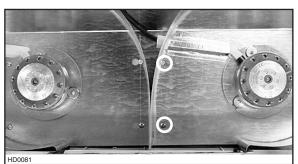
FOR P8 DUAL BLOWER UNIT, ENSURE THE IMPELLERS ARE CORRECTLY INSTALLED; THE HOOD WILL NOT WORK PROPERLY IF REVERSED. Both impellers are different in the dual blower, one rotates clockwise and the other counterclockwise. Each wheel and motor have an arrow and a number on them, you have to match them correctly (see drawing at right).
