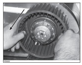
Install screws into the location as shown in the pictures below (P5 or P8 blower). Do not tighten screws down fully, leave a 1/8" gap. Hang blower unit onto blower plate (screws through the large part of the keyhole). Slide the blower to its position (screws in the small part of the keyhole). Tighten the screws.
