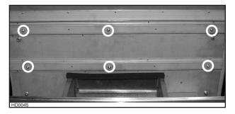
Secure the blower by installing 2 more screws into the locations shown in the pictures below (P5 or P8 blower). Reinstall impeller(s) and cover.
