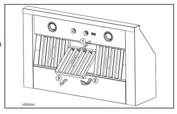
Remove bottom panel both retaining screws. Set bottom panel and screws aside.
