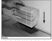
Inserting deviator into hood vertical opening.
