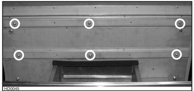
Secure the blower by installing 2 more screws into the locations shown in the pictures below (P5 or P8 blower). Reinstall impeller(s) and cover.
