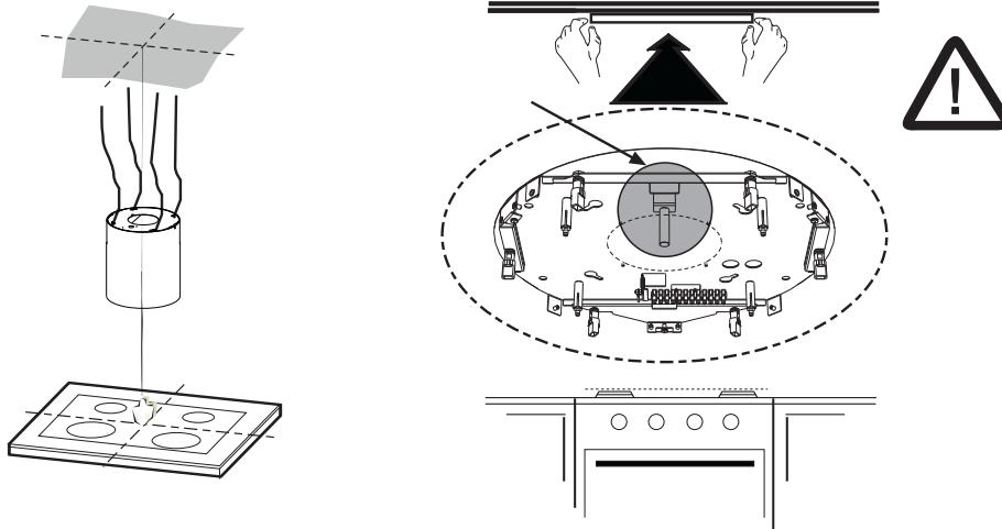
Use a plumb-line and mark the center of the cooking surface on the Support Ceiling.
