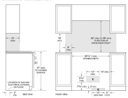
\*Without ventilation hood, 42\* (1067) minimum clearance countertop to combustible materials, charbroller requires non-combustible materials. NOTE: Shaded area above countertop indicates minimum clearance to combustible surfaces,
