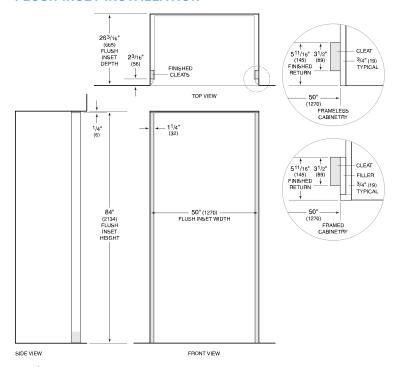
NOTE: 31/z\* (89) finished returns and shaded areas will be visible and should be finished to match cabinetry. Shaded line represents profile of unit with 3/a\* (19) panel.
