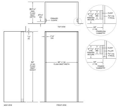
NOTE: 3<sup>1</sup>/2' (89) finished returns and shaded areas will be visible and should be finished to match cabinetry. Shaded line represents profile of unit with <sup>3</sup>/4" (19) panel.
