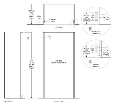
NOTE:  $3^{1}/2^{\circ}$  (89) finished returns and shaded areas will be visible and should be finished to match cabinetry. Shaded line represents profile of unit with  $3^{1}4^{\circ}$  (19) panel.
