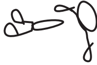
Wire clip (2) (for securing Drain hose joiner)
