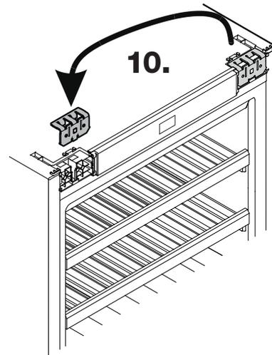
10. Remove the upper retaining bracket and transfer to the opposite side.
