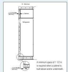
This is a fully integrated refrigerator-freezer which means that it is fully enclosed by a kitchen cabinet. This type of cabinet must be carefully constructed using the correct dimensions and it must provide suitable ventilation to ensure proper appliance operation.
