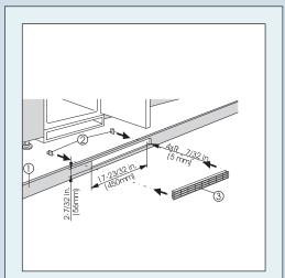
Ventilation through the cabinet base at the bottom can be achieved by installing the provided ventilation grille (3) or via a ventilation opening of at least 31 in.<sup>2</sup> (200 cm<sup>2</sup>).
