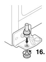
**16.** Tilt appliance slightly backwards, insert pin and attach using the adjustable foot.
