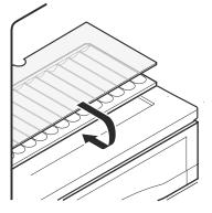
The cavities in the plate ensures secure placement of the bottles.
