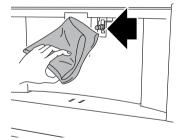
(5) Remove the milk container and clean the steam connection nozzle with a sponge.
