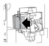
6 After cleaning, replace the infuser by sliding it onto the internal support and pin at the bottom, then push the PUSH symbol fully in until it clicks into place.
