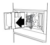
4 Press the two coloured release buttons inwards and at the same time pull the infuser outwards.
