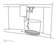
⑥ PLACE 2L CONTAINER UNDER SPOUTS, press TO FILL FILTER: Container has to hold at least 17 fl.oz. Delivery begins and stops automatically. The ௵ symbol appears on the display alongside the time to indicate that the filter has been enabled.
