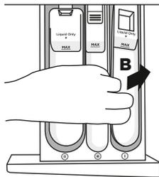
Removing the Pre Wash liquid detergent compartment
