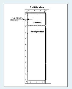
Do not restrict the air flow. The opening can either be directly over the appliance 1, above the cabinet and below the ceiling 2 or through a vent installed in a soffit 3.
