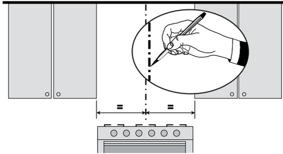
Draw a vertical line on the supporting wall as high as practical, at the center of the area in which the hood will be installed.
