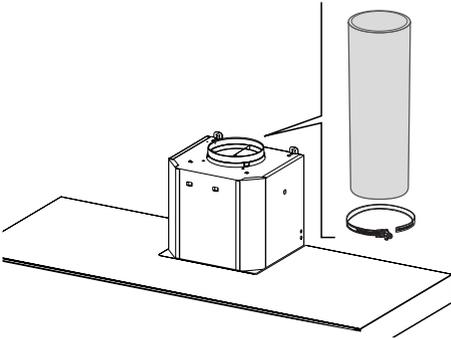
Only for the recirculation version, connect the hood to the Air outlet.
