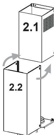
Slightly widen the two sides of the the lower chimney hood and hook them between the upper section and the wall, making sure that they are properly housed.
