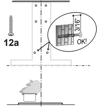
Insert the two screws 12a supplied with the hood as shown and do not tighten all the way to wall leaving 3/16" of the screw heads exposed.
