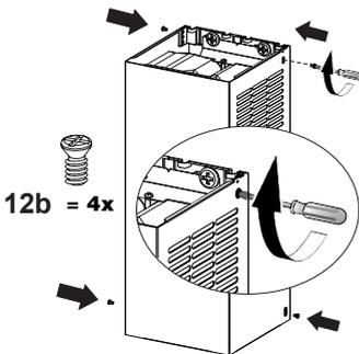
Secure the sides to the brackets by using the 4 screws 12b.
