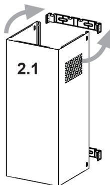
Slightly widen the two sides of the upper chimney and hook them behind the brackets 7.2.1, making sure that they are well seated.
