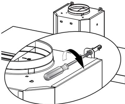
Tighten the 2 screws 12c as shown.
