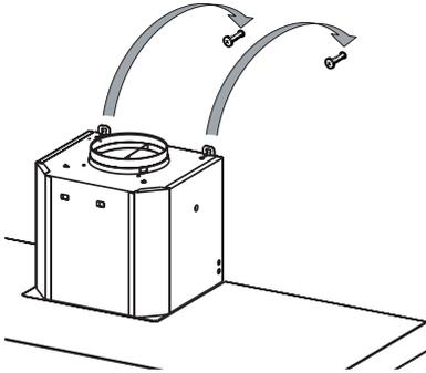
Hook the hood body onto the two screws as show.
