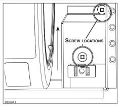
2.Install wire clamp (included) on top of blower box. Attach the adapter/damper to the blower box using 4 no. 8 x 3/8" quadrex screws (included). Remove tape on damper. (Angle brackets not illustrated to ease understanding).
