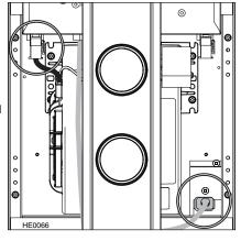
3. Remove the 4 screws retaining the blower box. Lift hood and set aside with screws.
